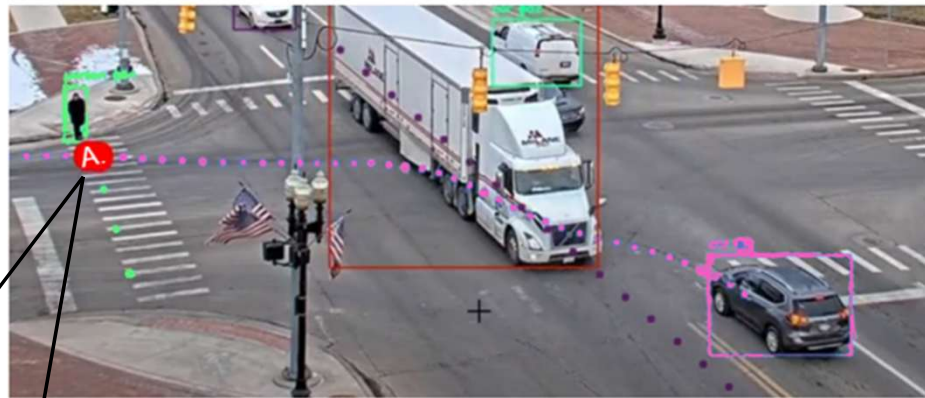
Figure 5.12: Downtown Coldwater, MI, USA traffic camera: Trajectory prediction and real-time overlap verification
