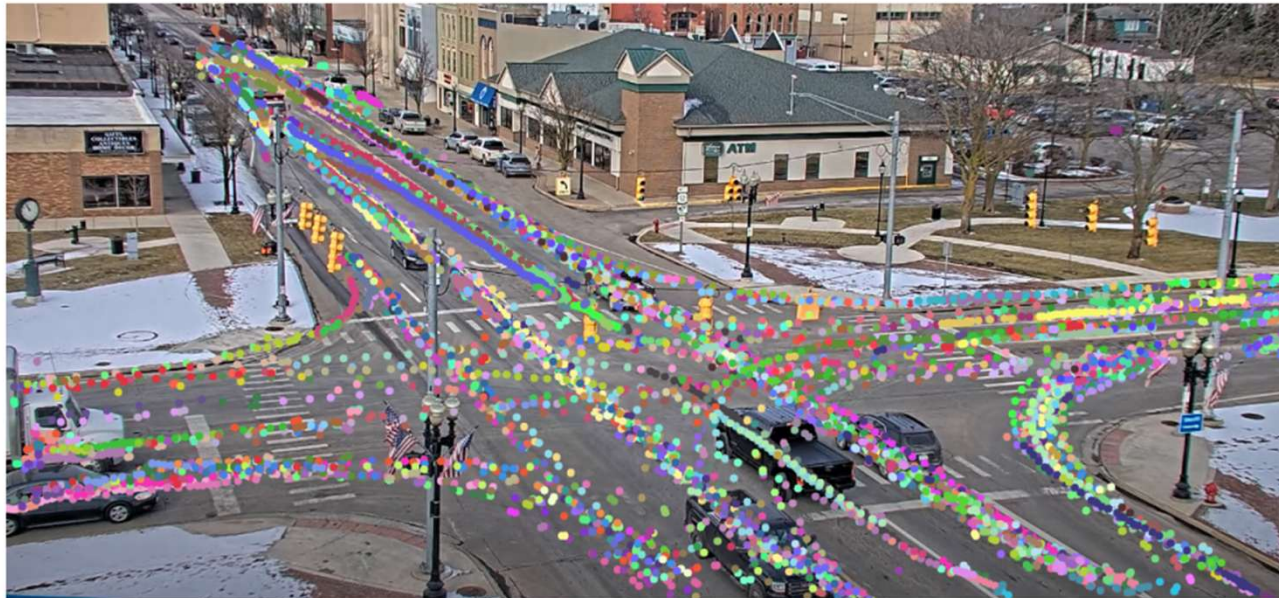
Figure 4.2: Downtown Coldwater, MI, USA traffic camera with trajectory visualization over 5 minutes
